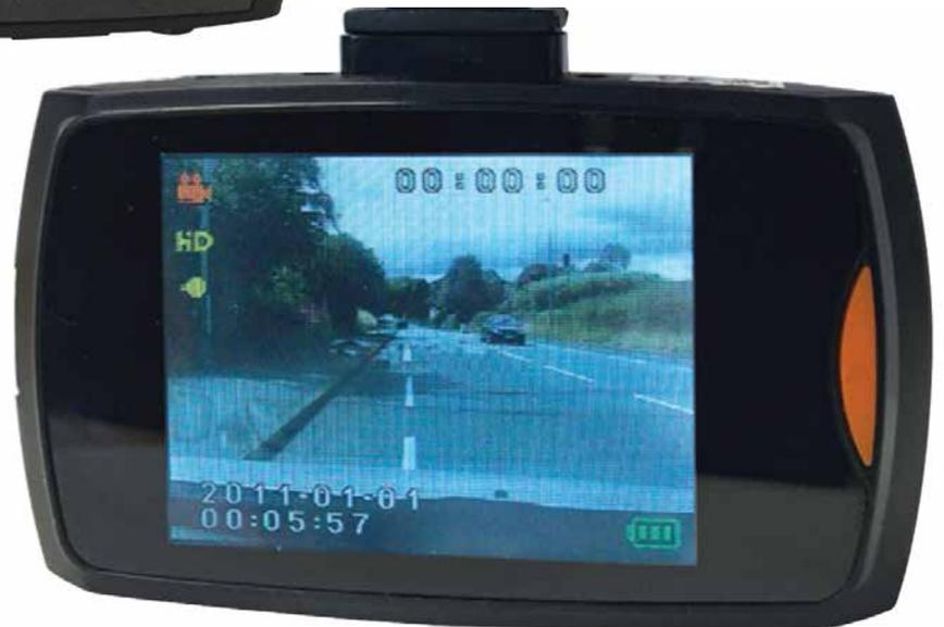
**Please note:** The internal battery for this Dash Cam is for playback and storing the system settings only. The Camera must be powered by the 12V power cable supplied or hard wired to the vehicle power supply to record any journeys.
